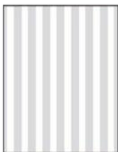
Hazard warning paving corduroy hazard warning surface
